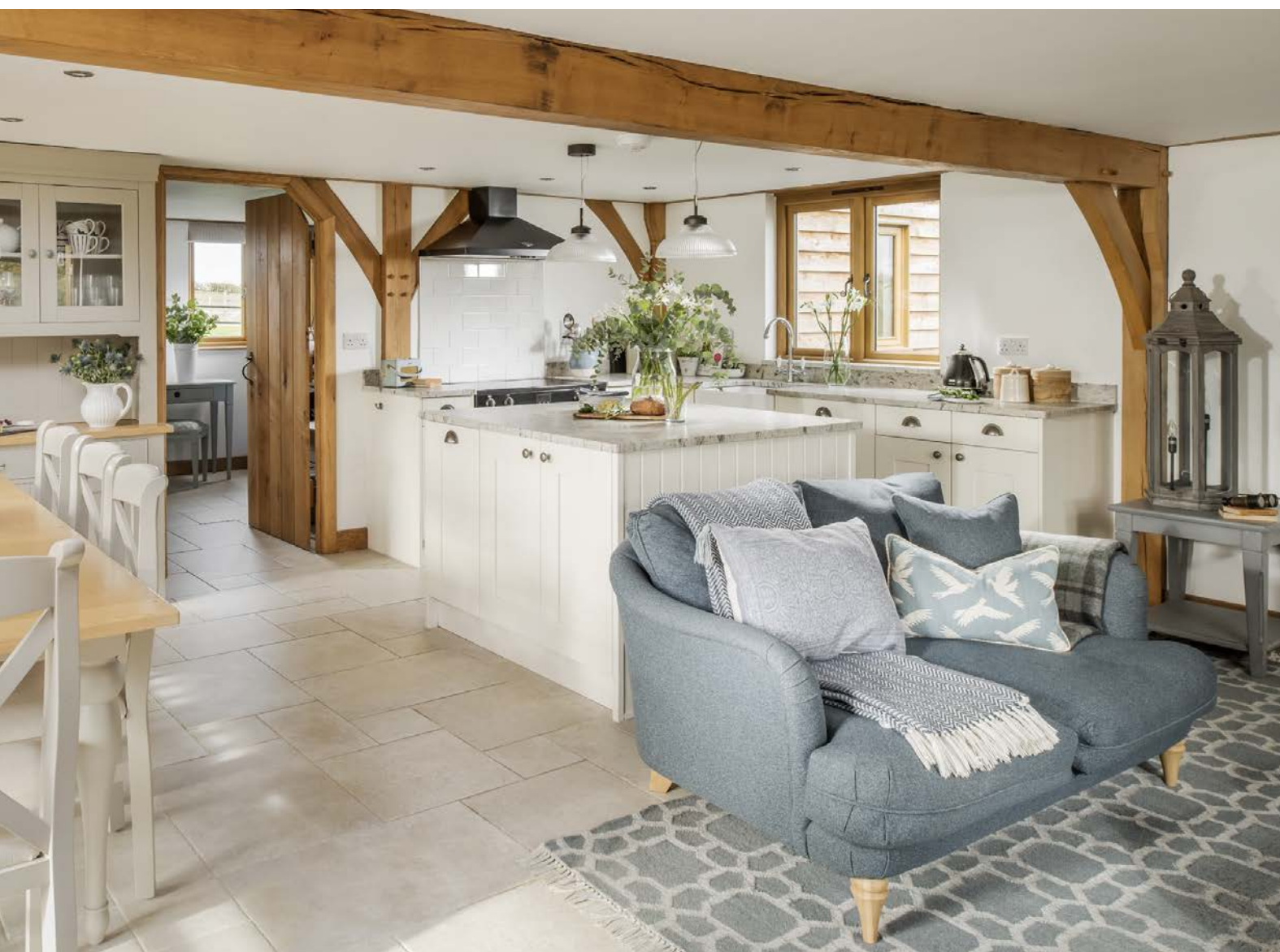
Below This open plan kitchen has large double casement windows with a trickle vent, meeting building regulation requirements. Both windows open. These windows can also be designed to have one fixed window and one open window, or both windows fixed dependent on your requirements for the space.
